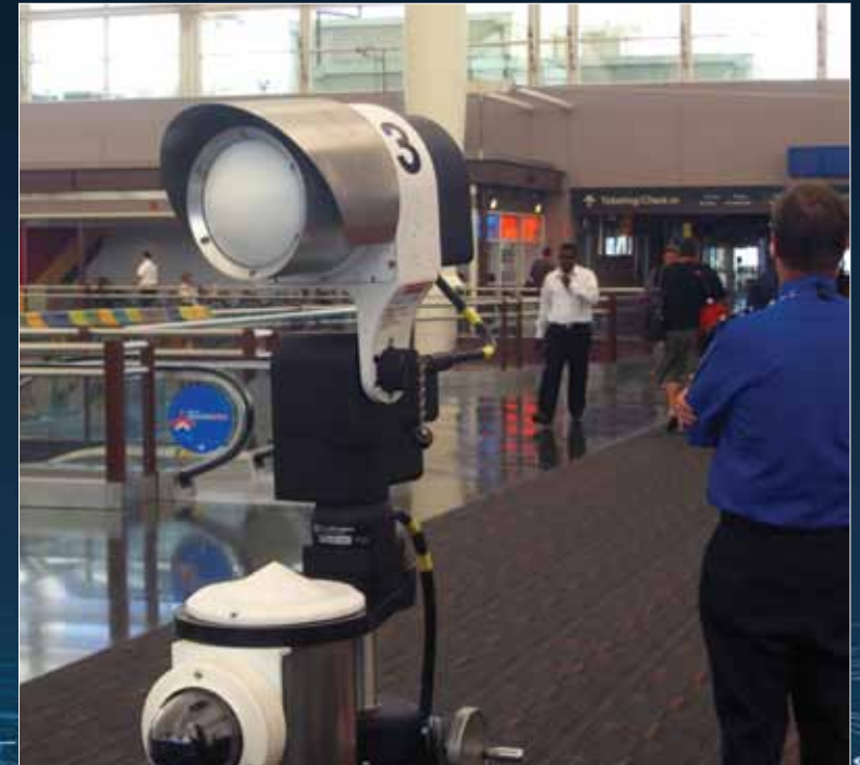
The PTU-D300 provides precise pointing for TSA security applications.
