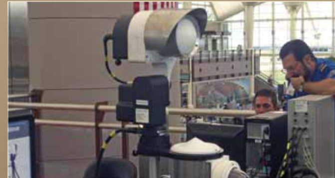
The PTU-D-300 is a key component in Qinetiq's stand-off detection system for the TSA.
