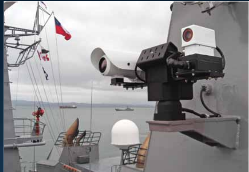
The PTU-300-ISM positioning an Optical Tracker on a Chilean Navy vessel.
